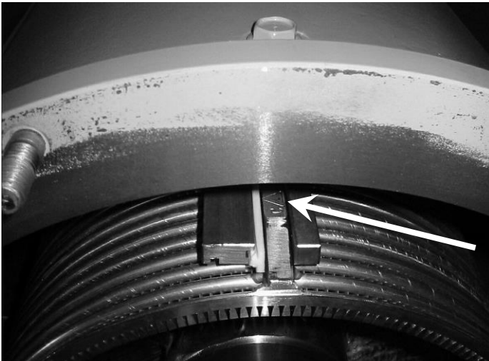
Fig. 13-10 screen installation position, stamped triangle at top and toward the front of the separator
