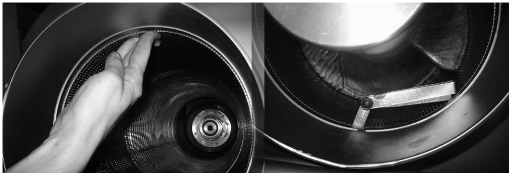
Fig. 13-11 Movable screen in the separator, inspection of the floating capacity by hand (left)
