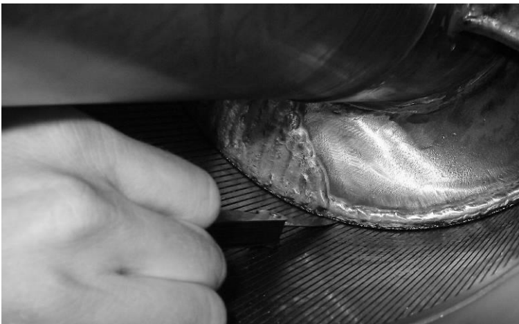
Fig. 13-15 Measuring of the working gap between the screen and the auger; the gap is measured on the bottom side of the screen while the machine is at rest. The measurement yields two times the working width because the screen rests on the top of the auger when the machine is not running.
